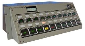
All switches are DPDT providing a total of four contacts (2 NO and 2 NC). Each processor board uses one NO and one NC contact to provide redundant switch state information. A fault is reported if the switch remains in an illegal state for any length of time. The second pole goes to the second processor board. If there are more than two processor boards, they alternate. Each
