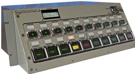
All switches are DPDT providing a total of four contacts (2 NO and 2 NC). Each processor board uses one NO and one NC contact to provide redundant switch state information. A fault is reported if the switch remains in an illegal state for any length of time. The second pole goes to the second processor board. If there are more than two processor boards, they alternate. Each processor board contains isolation diodes to localize any fault that might occur in the board.
